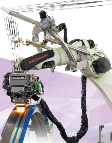
TFL uses thermoset prepreg slit tape. 16 spools can be installed in the creel box as standard. Those tapes are delivered to the head at optimized tension control. TSUDAKOMA's tension control technology was originally developed for textile machines. High quality slit tapes can be produced using our TPS prepreg slitter.
