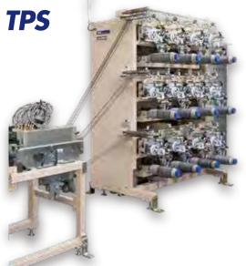
Optional off-machine winder for TPS prepreg slitter to rewind narrow slit tapes with widths such as 1/8", 1/4", 1/2", 1". Bobbin traverse system is adopted. Each tape tension is controlled individually by TSUDAKOMA's original tension control technology. Liner film unwinder is employed to rewind thermoset prepreg tape, used on the Automated Fiber Placement (AFP).
