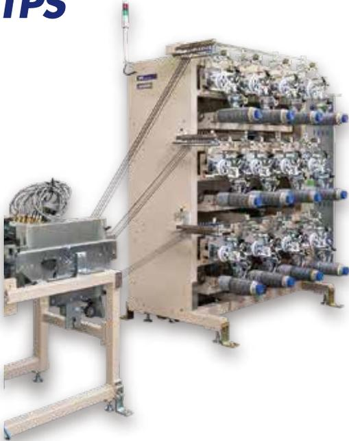
Optional off-machine winder for TPS prepreg slitter to rewind narrow slit tapes with widths such as 1/8", 1/4", 1/2", 1". Bobbin traverse system is adopted. Each tape tension is controlled individually by TSUDAKOMA's original tension control technology. Liner film unwinder is employed to rewind thermoset prepreg tape, used on the Automated Fiber Placement (AFP).
